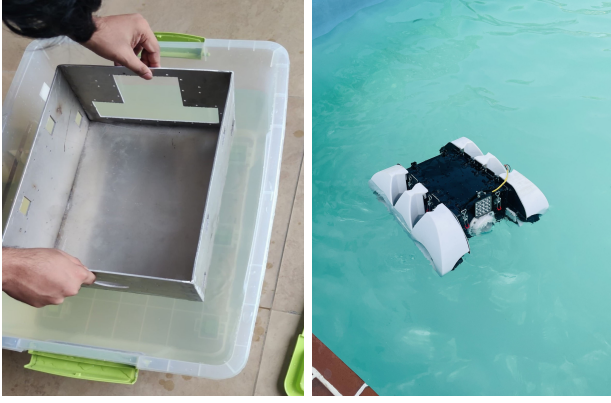
(a) Checking tiny leaks (b) Floating Water tests
