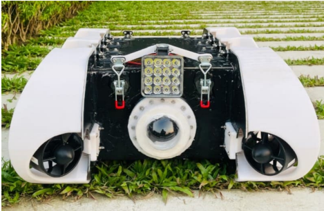
Fig. 11: After Installing Camera and Lights
